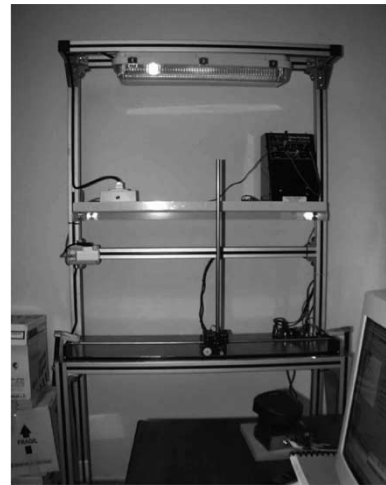
Fig. 2. Inverted pendulum adapted to the remote experimentation.
