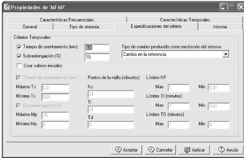
Fig. 9. Specifications for a tuning by settling time and/or maximum overshoot.
